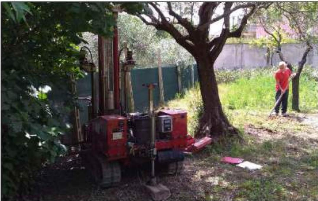
Foto 9 – Prova penetrometrica DPSH 04
